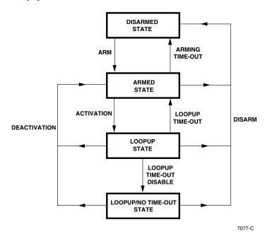
Figure 102-1. Loopback Operation State Diagram
